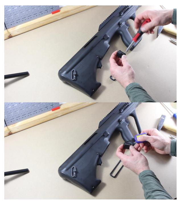
Put the two parts of the Case Deflector together:
