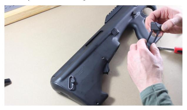
Place the Case Deflector in the ejection port with the wedge shaped piece at the rear:
