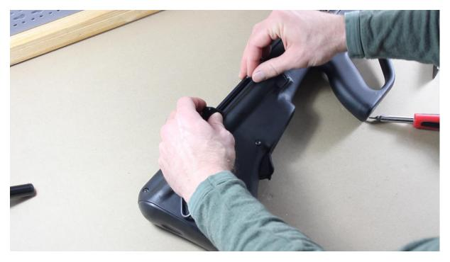
Insert and alternately tighten the two screws until the Case Deflector sits firmly in the ejection port.
