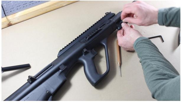
Alternately tighten the grub screws until the rail is firmly seated.
