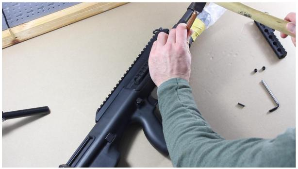
Apply thread locker to the grub screws and tighten until they flush with the rail:
