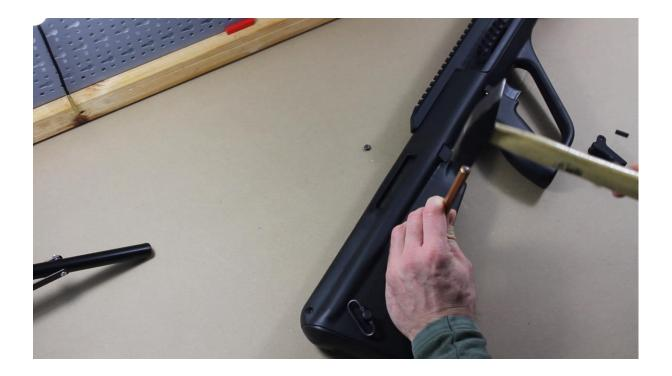
Insert original spring in the Corvus Defensio Enhanced Release Button and fix it with mounting pin (included). The short end of the spring must be in the Release Button.
