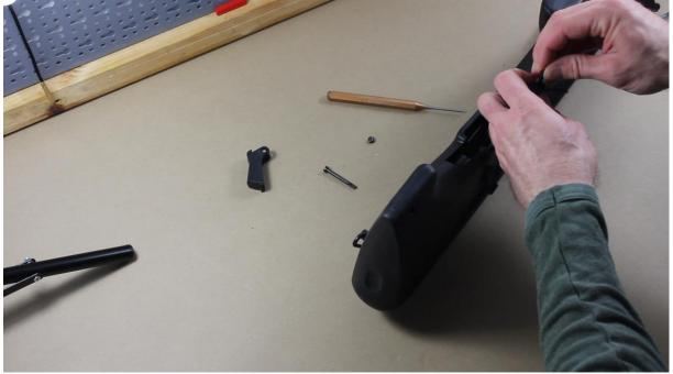
Put the assembled (spring and included mounting pin) Enhanced Magazine Release Button into the AUG stock and knock in the bolt/screw (this motion pushes through the included mounting pin that holds the spring in place).
