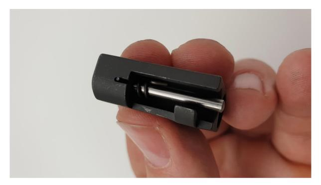
Slide the base with the pin onto the charging handle mount of the receiver.
