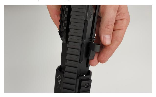
Push/pull the other end of the spring over the charging handle mount of the receiver using the small screwdriver or allen key.
