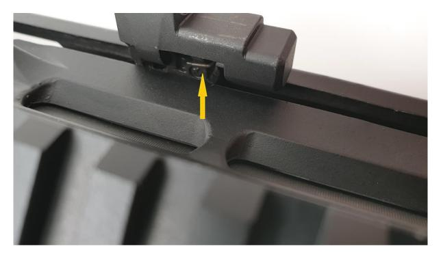
Place the cover and slide through the connecting screw.
