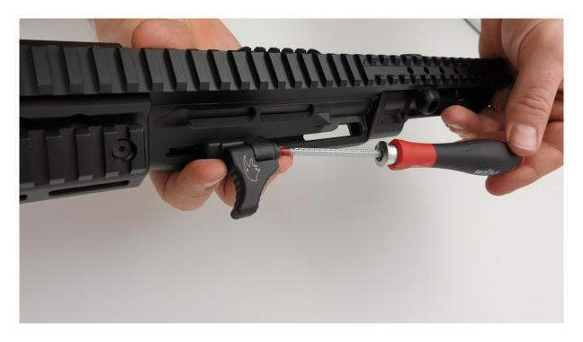
The charging handle can be adjustet to any desired angle now.
